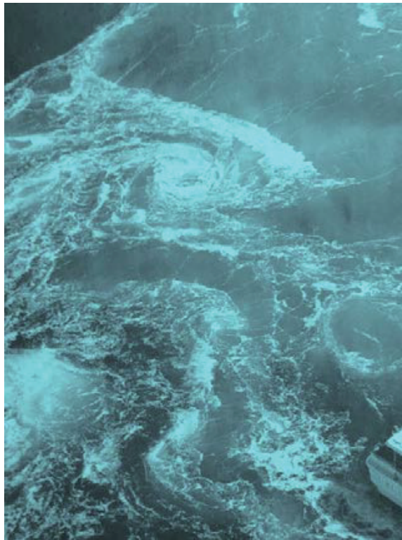
Fig.1(a) Aerial photograph of large-scale vortices in Western port, Victoria, Australia. After Pollock, 1973.
